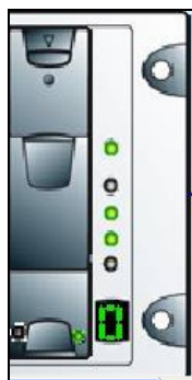
Figure 26 - Ops Panel for 14 bay on front of chassis
