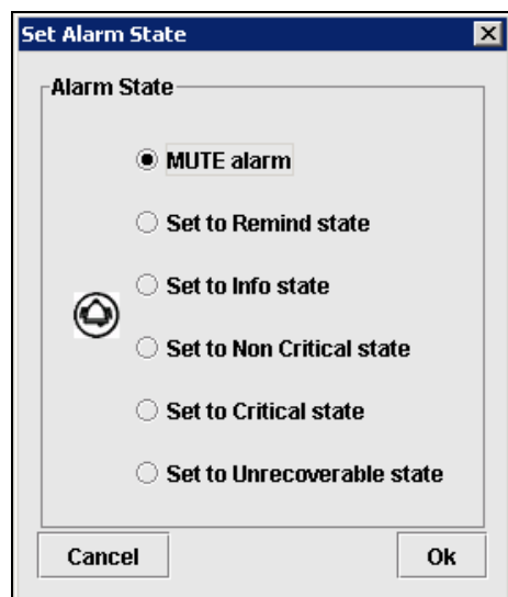
Figure 35 - Set alarm state shown muting an enclosure
